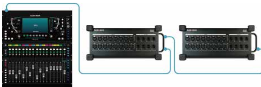
SQ + 2 x DX168 32 remote inputs + 16 remote outputs
