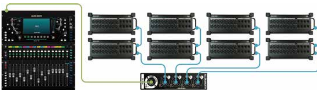
SQ + DX Hub + 8 x DX168 128 remote inputs + 64 remote outputs
